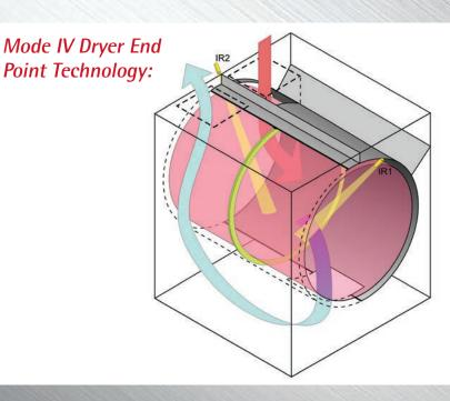
Milnor uses two infrared sensors in conjunction with inlet/outlet temperature profiles to determine accurately when the goods are dry.
