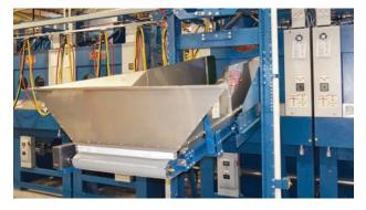
Milnor dryers are pass-through machines that load at one end and discharge at the other. They form an integral part of an automated batch laundry processing system, along with a PulseFlow<sup>®</sup> batch washer or continuous batch washer, an extraction system, and transport conveyors.
