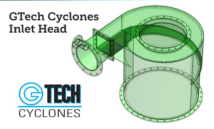
There are two main types of inlet heads that are widely used, Tangential and Scrolled Evolute. The Tangential inlet dates back to 1939 when the Dutch States Mine (DSM) started investigating the use of cyclones for cleaning coal. The Scrolled Evolute is a more recent development and has been found to offer several key advantages over the tangential Inlet.
