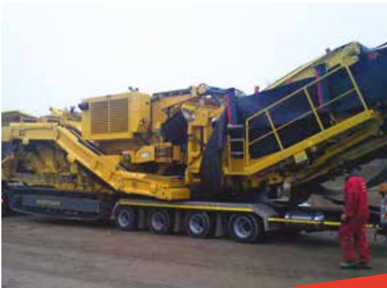
The Dolly transport system reduces weight, length and height and the need for permits
