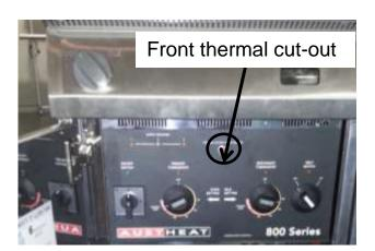
When the thermal cut-out has tripped, a red button on the device will protrude out from the panel where it is located. This protrusion is an indication that the cut-out has tripped. If the thermal cut-out has tripped, it indicates that there is an underlying problem that has caused the oil to reach a dangerous temperature.
