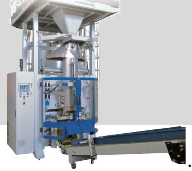
The Ilerbag V is a vertical form fill & seal for large bags where the P.E. film is taken from the roll and formed into the bag shape then filled & sealed. This is ideal where long runs of the same bag are required
