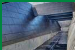
Wear liners to suit material being handled
