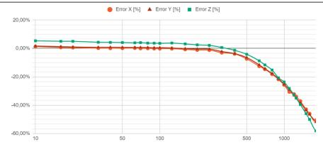
Figure 1 - IOLITEi 3xMEMS-ACC frequency response (Range: 2g, SR: 4 kS/s)
