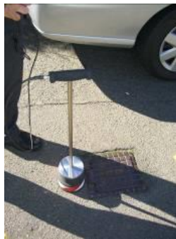
Fig. 25 Pin Pointing with a Geophone
