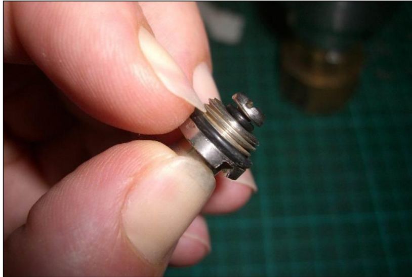
Fig. 61 removed Hydrophone Bleed Valve
