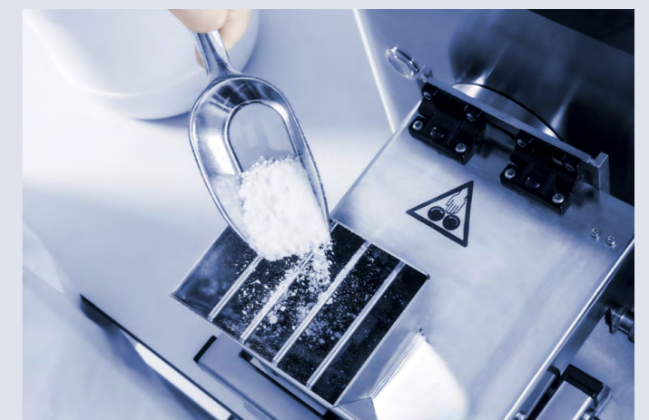
Mixer for characterization of silica and other powdery materials
