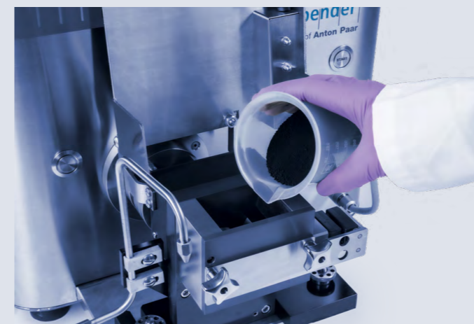
Mixer for characterization of industrial carbon blacks
