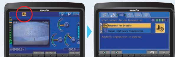
Aftertreatment device regeneration screen
