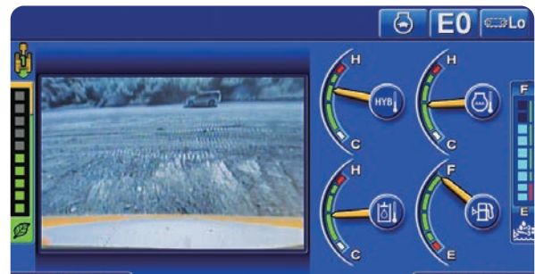
Hybrid system temperature gauge
