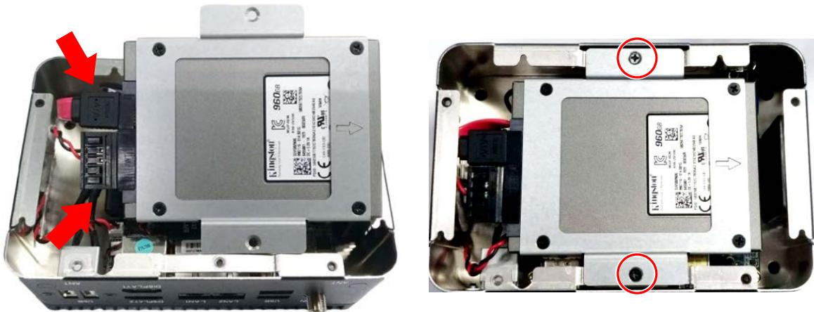
5. Slide back the bottom cover and then screw the cover back to the system.
