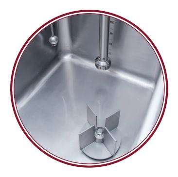
The spinner speed varies automatically depending on the quantity of mix, that is measured by a floating sensor placed inside the tank; minimum and maximum charges are processed with the same efficiency, to grant the best possible heat transfer and to avoid foaming.
