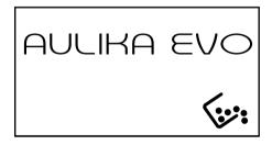
If the drawer is not emptied after several brewing cycles, the machine will stop and the display will show:
