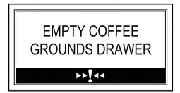
In this case, the machine does not allow beverages to be dispensed. In order to dispense beverages, the coffee grounds drawer must be emptied of used coffee.
