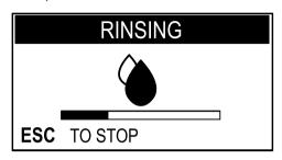
The progress bar indicates that the machine is performing the rinse cycle of the system.
