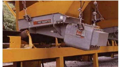
Large Vibratory Feeders meter stone to a belt conveyor from a hopper.
