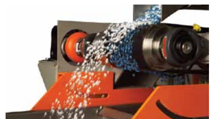
Magnetic roll separates co-molded plastic regrind containing PolyMag™ metallic additive.
