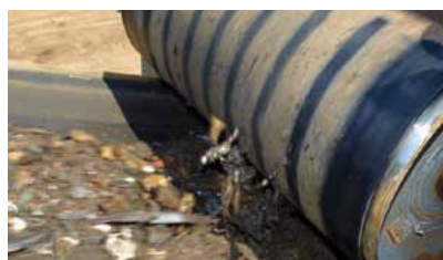
Auto shredders use Magnetic Pulleys to separate ferrous metals on Scavenger Belt.
