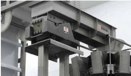
Sanitary Vibratory Feeders present products to weigh scales in packaging applications.
