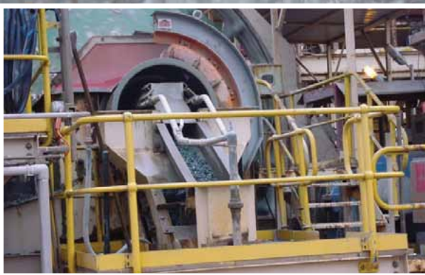
▼ Trunnion Magnet removes broken ball fragments on a Ball Mill in Chile.
