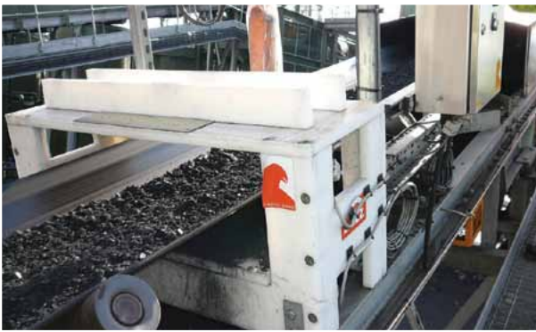
▼ MetalArm Metal Detector scans for metal tramp in coal mine operations.
