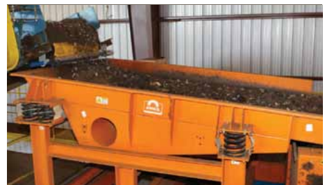
Mechanical Feeder presents an even flow of material to an automated sorter at a scrap yard.
