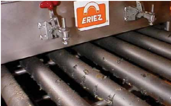
▲ Grain mill uses Xtreme Rare Earth Grate Magnets to remove metal contaminants.
