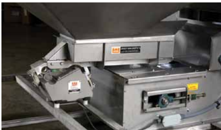
High Deflection Feeders are designed to feed difficult materials like powders as well as sticky and leafy products.
