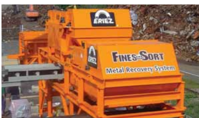
FinesSort® recovers small ferrous from waste at a scrap yard in Tennessee. Powerful Rare Earth Magnets recover virtually all ferrous metal from crushed automobiles and other scrap.
