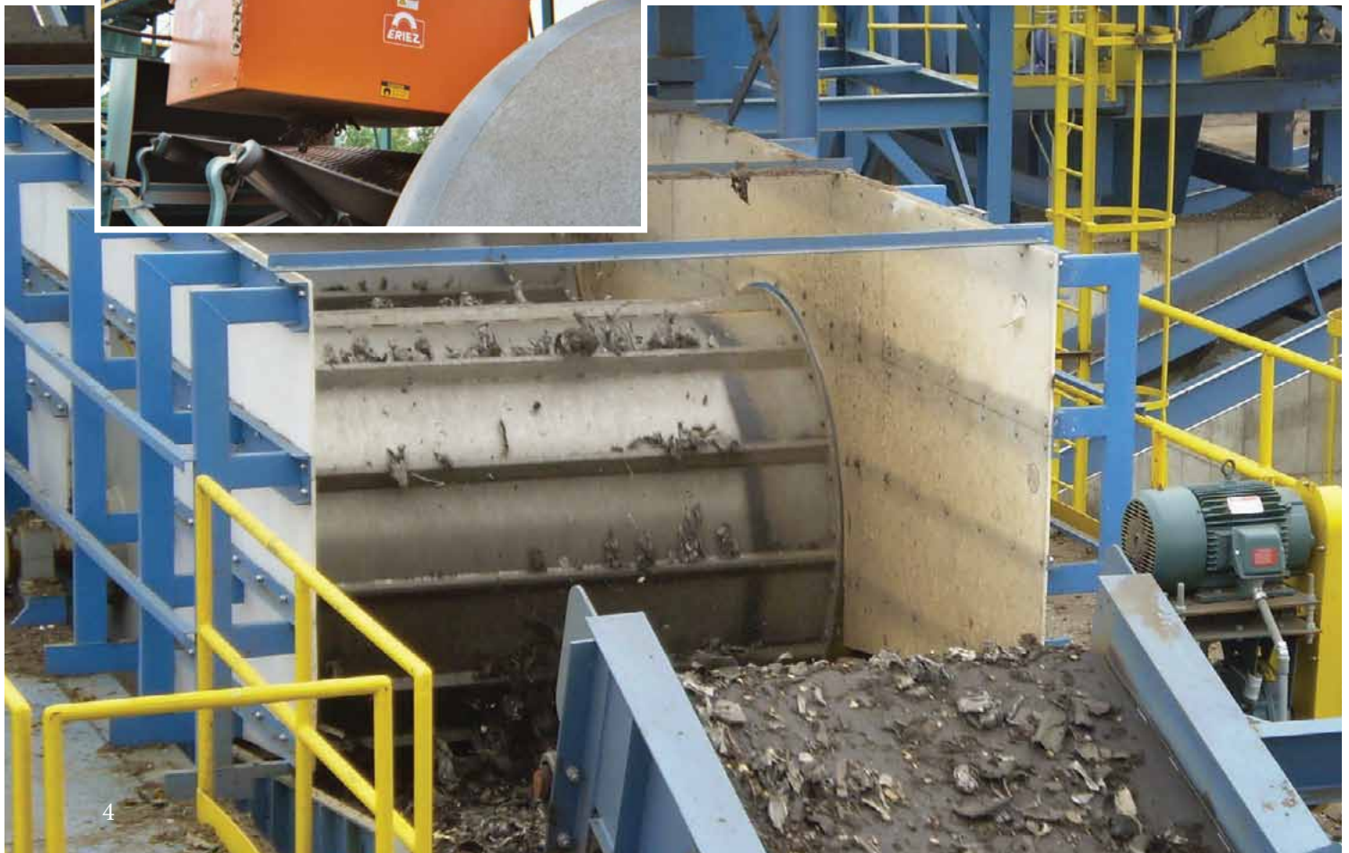
▼ Scrap Drum Magnets separate ferrous metals at an auto shredder in Ohio.
