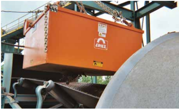
▼ Electromagnet removes tramp metal at an aggregate plant in Pennsylvania.
