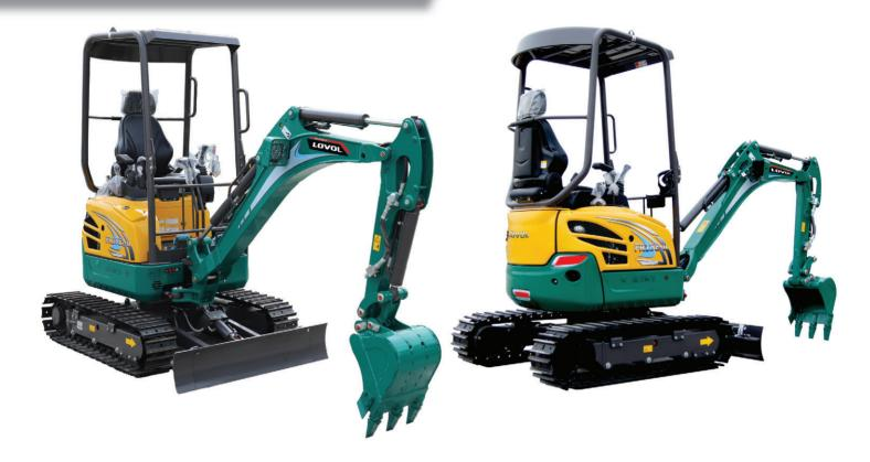
The LOVOL 1.8 tonne ALFA series excavator features a Yanmar Engine with mechanical fuel pump, so no ECU, eliminating problematic electrical items. Nabtesco hydraulic system with pilot oil operated joysticks for precision and control.
