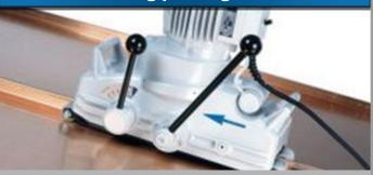
Double standing pleating machine to fold double standing seam of profile plates in a single operation. For turned-up metal sheets, 2 seaming operations are necessary. The seam prfile height is infinitely variable from 20-40 mm, depending on the profiler or turn-up height.
