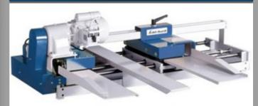
Edge bending machine for parallel plates, with both edges being Double standing pleating machine to fold double standing seam folded up in a single operation. Turn-up height between 25 – 60 of profile plates in a single operation. For turned-up metal mm and intake width of 350–1,000 mm, infinitely adjustable.
