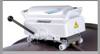
Universal folding machine produce angular and double standing seams in a single operation, for straight or arched profile plates from a radius of 600 mm. Adjustable for seam profile heights of 25 and 38 mm.
