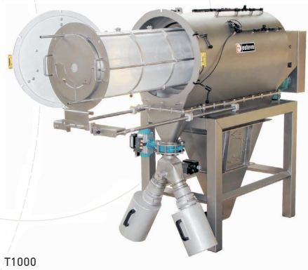
T1000 Mesh of 600 microns. Equipped with a slide for quick inspection of the sieve. By-pass selection of foreign particles.
