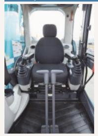
The new 'Big Cab' provides a roomy operating space with plenty of legroom, and the door opens wide for easy entry and exit. As well as giving a wide, open view to the front, the cab has increased window areas on both sides and to the rear, for improved visibility in all directions.
