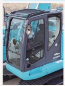
The newly developed, ROPS (Roll-Over Protective Structure)-compliant cab clears ISO standards(ISO-12117-2: 2008) and ensures greater safety for the operator should the machine tip over.
