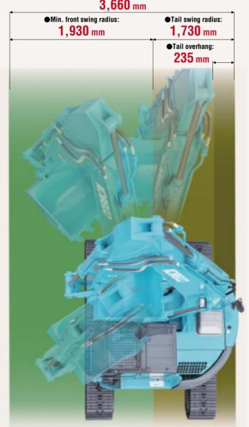
\*"Working distance" equals the sum of the minimum front swing radius and tail swing radius.
