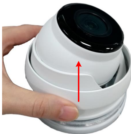
Remove the Outer Housing
