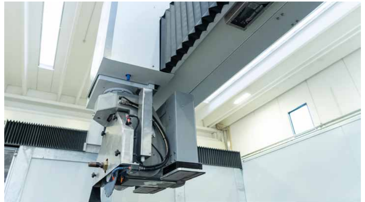
CAMERA: system to obtain the images from the working table, it permits to accellerate the pieces positioning and notice possible bugs on the slab
