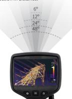
Both T300 and T600 have ultra-high thermal sensitivity of 35mK, highlighting more temperature details and finding out the potential risks that are difficult to find by low-sensitivity equipment during inspection
