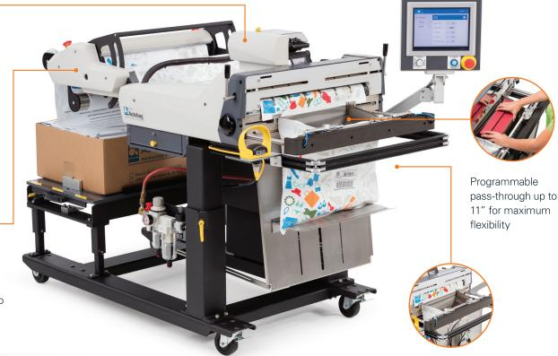
Unobstructed access minimizes guarding for easy access to the open bag
