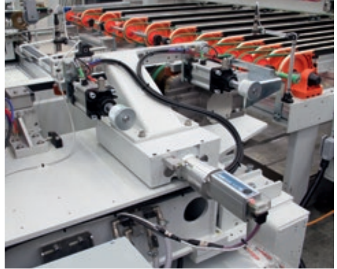
The automatic adjustment of the reference line to remove the glass according to the thickness prevents the operator from intervening manually.
