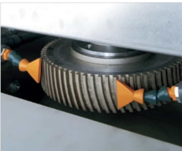
Oscillating peripheral grinding wheel
