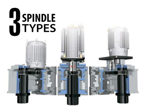
Inline Drive The standard configuration for most Haas 40-taper VMCs is an inline direct-drive spindle that is coupled directly to the motor to provide excellent surface finishes and greater thermal stability. The inline spindle is available in 8100-rpm, 10 000-rpm, and 12 000-rpm configurations.
