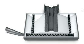
Triple Auger VF-1 and VF-2 machines (all models) are available with a high-volume chip-removal system comprising dual side augers to transport chips to the front of the pan, and a primary chip auger to discharge the chips from the machine.
