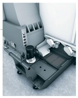
21 bar or 69 bar Through-Spindle Coolant Through-spindle coolant uses an auxiliary pump to supply coolant through the tool, directly to the cutting edge. This increases tool life, allows higher cutting speeds, and clears chips during deep-hole drilling and blind-pocket milling. Two systems are available. One provides up to 21 bar to the cutting edge, and the other provides up to 69 bar. The 69 bar system includes the auxiliary coolant filter (described below).
