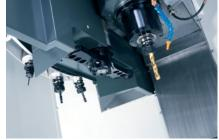
The DT-1's high-speed 20+1 tool side-mount tool changer swaps tools quickly to reduce noncutting time. The 12 000-rpm inline direct-drive spindle allows rigid tapping to 5000 rpm, with up to 4-times retract speed.
