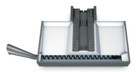
**Single Auger** All Haas VMCs are available with a single, auger-style chip conveyor that automatically removes chips from the machine, while compressing them and wringing out the coolant. For added reliability, the system reverses automatically if a jam occurs.
