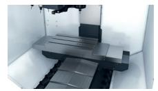
Steeply sloped internal sheet metal and available dual chip augers efficiently move chips to the rear of the DT-1 for discharge.
