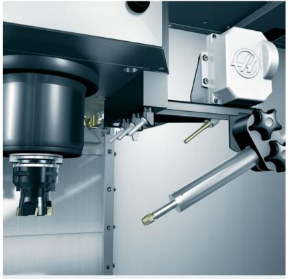
Automatic Air Gun Provides a constant blast of air to the cutting tool to clear chips during dry machining. Activated by M-code, the air gun can be programmed to turn on while the spindle is turning, or at the end of a cycle. Air consumption is 6 scfm.
