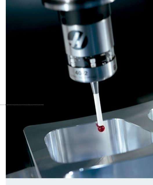
**Haas Wireless Intuitive Probing System** The Haas Wireless Intuitive Probing System (WIPS), with optical transmission for part setting, tool setting, and inspection, consists of the following elements:
