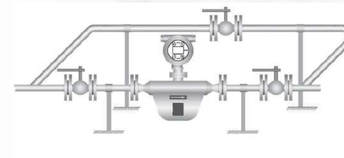
Horizontal Installation of V-Type Mass Flowmeter
