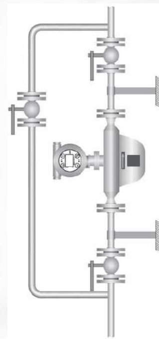
Flag Installation of V-Type Mass Flowmeter
