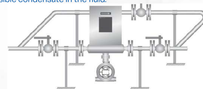
Inverted Installation of U-Type Mass Flowmeter
