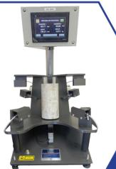
Concrete Test Cylinder Measuring Station
