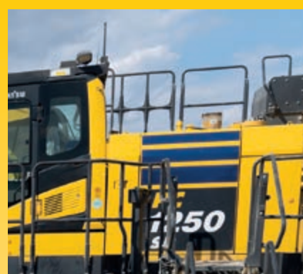
Hand rails and anti-slip plates
