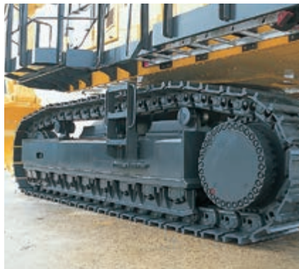
Full length track roller guards (optional)
