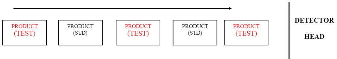
It is a failed test if any of the test packs are not rejected. If a standard pack is rejected the line must be stopped and the issue investigated e.g. timing of reject mechanism.
