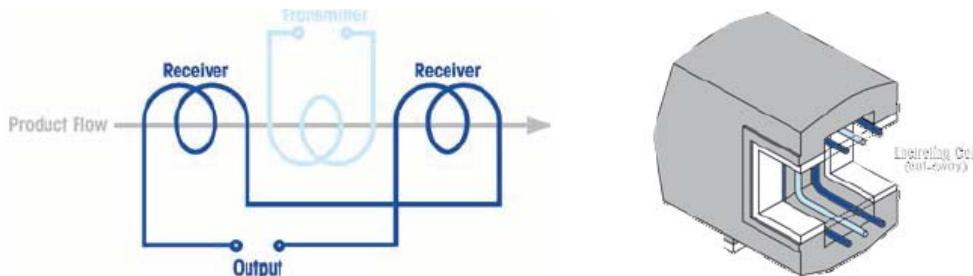
As much as we rely on metal detectors, as a means of quality control, they are still unable to detect every particle of metal passing through them. As with any measuring instrument, there are restrictions on accuracy and this varies depending on the application.
