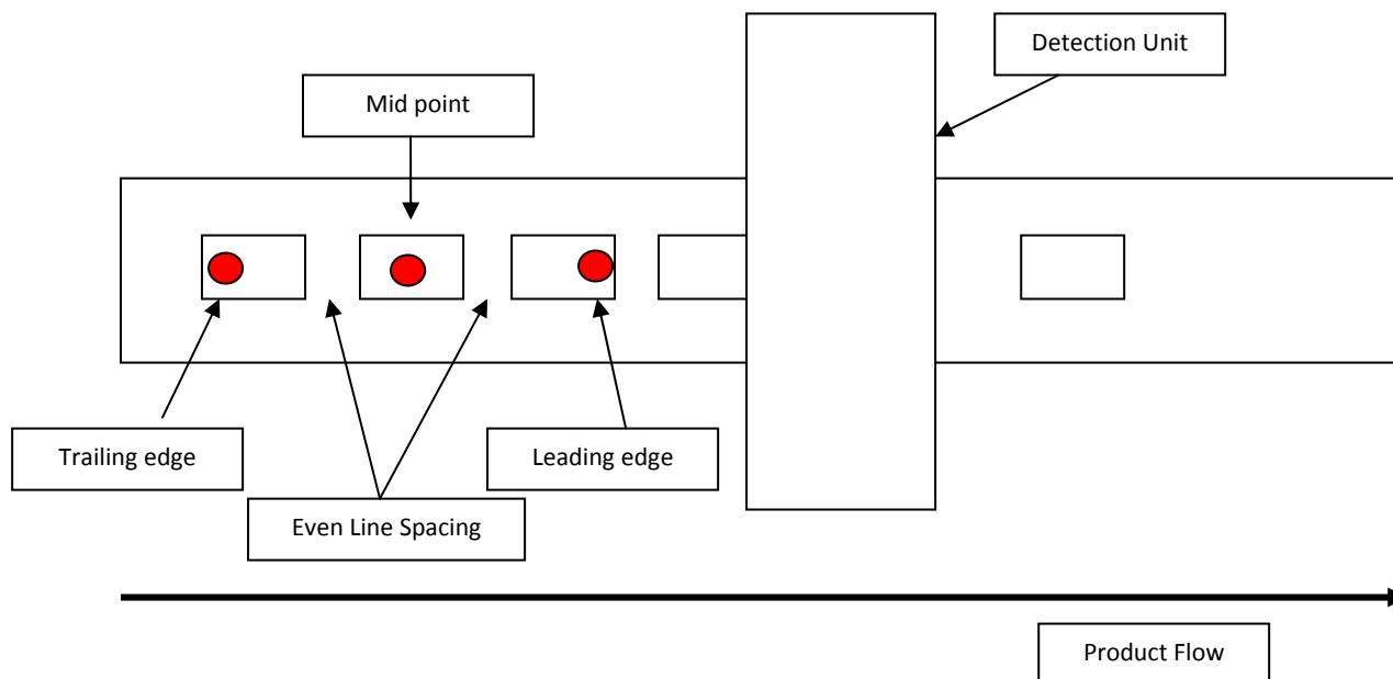
For Ferrous in Foil Detectors two test packs are required including two ferrous test pieces of the same size.
