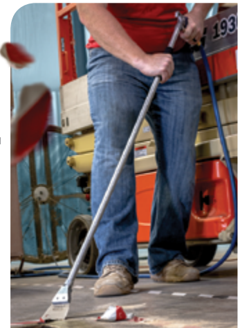
The Model 1244-36 scrapes and blows old tape off a concrete floor.
