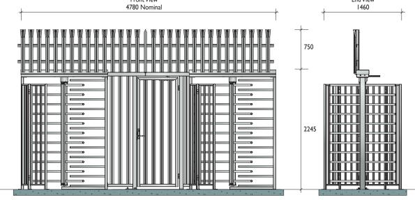
Leda full height turnstiles integrate with other access control systems and cater for a flow of up to 20 people per minute. Controllers can be configured to provide a range of functions (entry only / exit only / entry and exit). Recommended minimum for all concrete footings, 30MPa.
