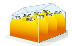
Infrared heating solution brings **comfort** directly to the end users level and limiting heat losses then generating **energy savings**. The SBM solution is efficient even for not insulated buildings with height from **4 to 25 m** or **outdoor heating**.
