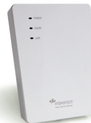
Area Control Gateway or Network Coordinator Relays Alerts to Application Software
