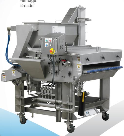
Breader designed for flour and fine granular free flowing coating materials
