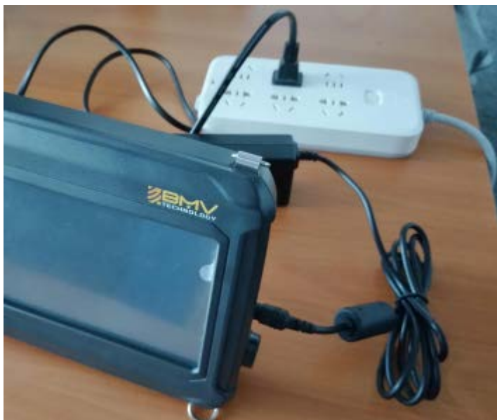
Figure 4-5 connection of power cable of the adapter
