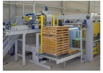
This system conveyors the bags up & slides them into position to form a layer. The layer is pressed on all four sides and the pallet is then raised and the layer is placed on the pallet. The layer top is pressed for form a flat surface to the next layer.
