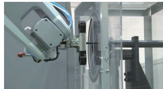
Sprue cutting of a CFRTMP molded item
