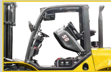
The easy to open hooks provide quick and easy access to the engine compartment
