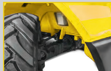
Oscillating steer axles allow all wheels to step over obstacles, whilst keeping the truck and load level
