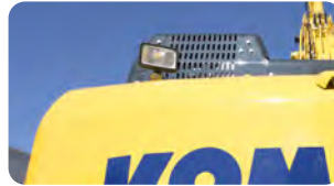
Additional Lighting Extra lighting on cab and counterweight for improved visibility.
