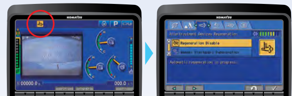
Aftertreatment device regeneration screen
