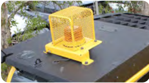
Rotating Amber Beacon Fitted with factory guard.
