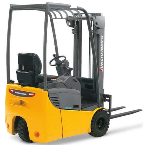
Load capacity: up to 1,500 kg
