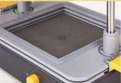
Airflow Control A super fine mesh made from pressed steel increases airflow to 3D shape
