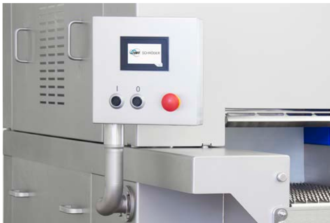
Standard touch panel for controlling the basic functions, including transport and needle rinsing function
