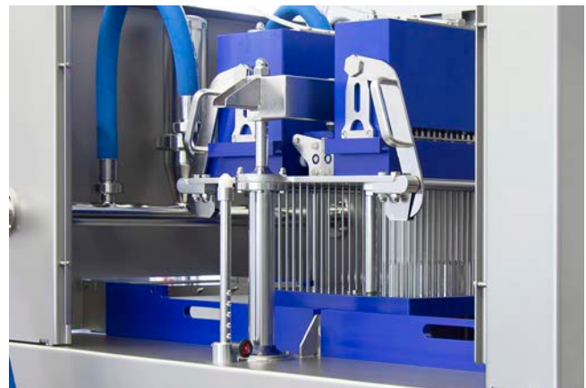
Injection and tenderizer head (right) with retraction block, injection needles with 2 mm, 3 mm or 4 mm diameter, tenderizer blade with ground tip (4 mm diameter)
