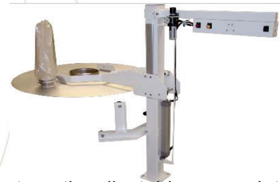
An automatic adjustable cover plate can be added for different size of bowls
