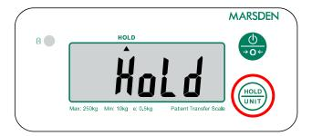
With a patient on the scale, press HOLD/UNIT. The display will show 'HOLD'. NB: Alternatively, you can activate the Hold function before the patient is on the scale.
