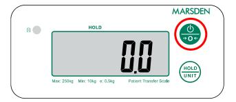
To switch the scale on, press the ON/OFF/ZERO button. When the display shows 0.0 the scale is ready to use.
