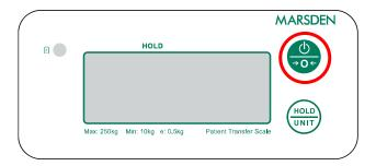
Press and hold ON/OFF/ZERO button for three seconds to power the scale down.
