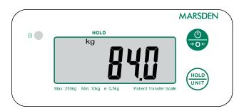
When the scale has determined the weight of the patient, a stable weight reading will show. This will remain on the display after the patient has left the scale.
