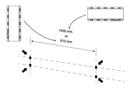
Use the Patient Transfer Scale and the hooks to determine the positioning of the hooks on the wall, and mark drill holes. Drill holes should be exactly 1400mm or 610mm apart, as per above.
