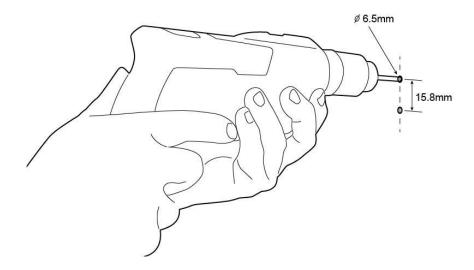
Affix the hooks to the wall using the screws and wall plugs provided, and use the plastic covers to hide the screwheads.
