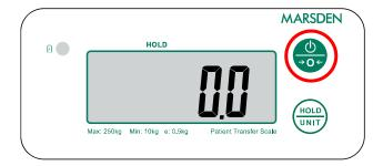
If for any reason the scale shows a reading other than 0.0 it can be reset to zero. Press the ON/OFF/ZERO button once and the scale will return to 0.0.
