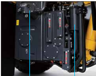
Hydraulic oil filter (Return) Brake cooling oil filter (Return)
