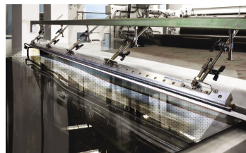
This 96" Long Gen4 Super Ion Air Knife cleans an acrylic sheet before protective wrap is applied.
