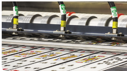
Gen4 Ionizing Points remove static from a card slitting operation.
