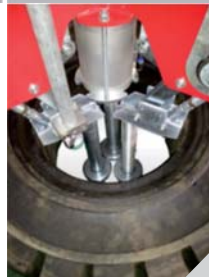
□ RA200 - Tyres Mandrel tooling with pneumatic inclination
