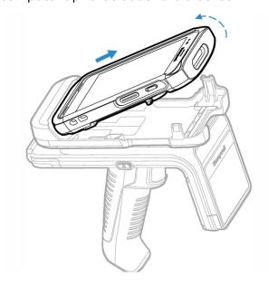
3. To remove the bracket, hold the handle with one hand and lift the bracket up from the RFID Reader with the other hand
