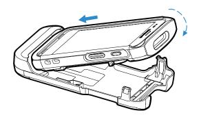
2. Align the bracket with the socket, ensuring that it is parallel, and press the two parts together firmly until they click into place.
