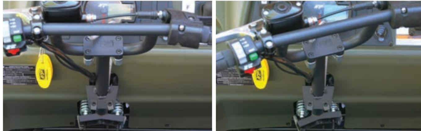
By adding a spring element between the handlebars and the brake system, we achieved a progressive dual-rate steering system.
