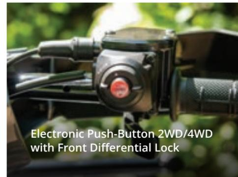
Electronic Push-Button 2WD/4WD with Front Differential Lock
