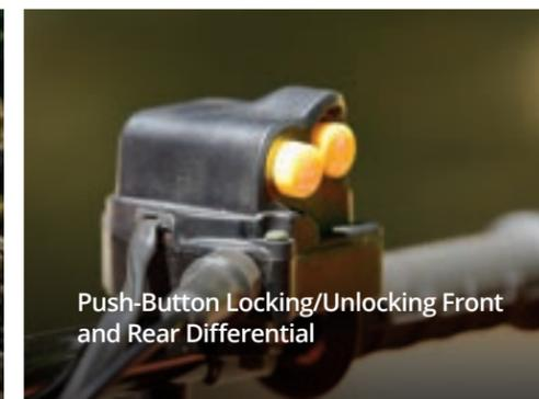
Push-Button Locking/Unlocking Front and Rear Differential
