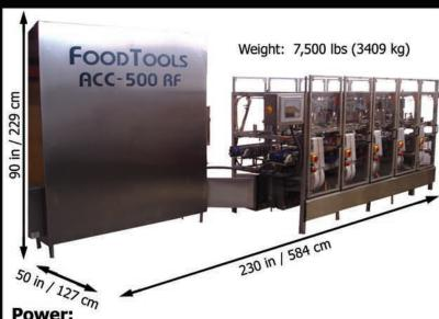
Compressed Air 40 CFM @ 90 PSI Electric 480V/60/3 Phase, 60A
