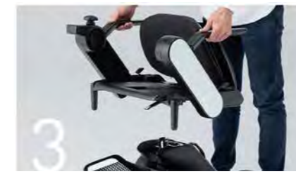
3 Pull the seat upwards.
